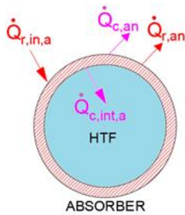
Fig. 2: Absorber tube heat fluxes
